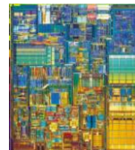
2001 Pentium 4 Processor 42 Million Transistors
