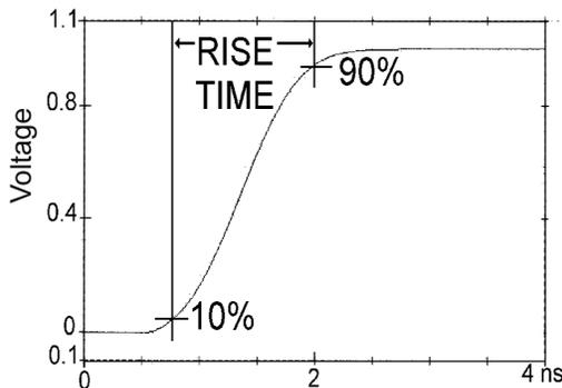
Figure 1: Step Response of 1 ns Risetime Gaussian
