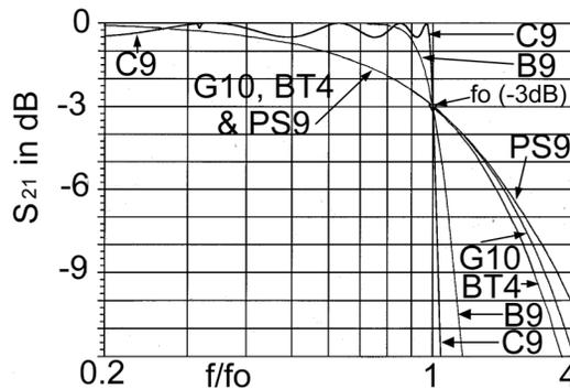
**Figure 4: Comparison of Insertion Loss in dB vs. Normalized Frequency ( $f/f_o$ )**
