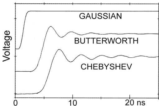
**Figure 3: Comparison of Step Response.  $f_o = 332$  MHz**
