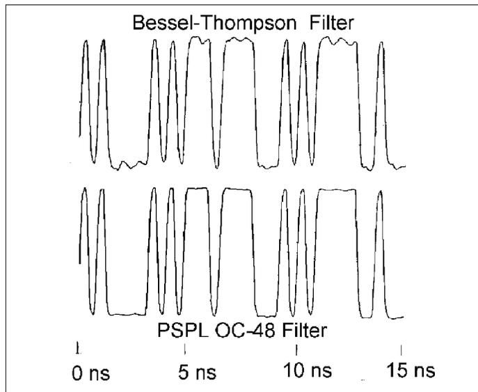
**Figure 11: Performance in a Mismatched Data System. A Randomly Selected 15 ns Segment of 2.5 Gb PSRB Data.**
