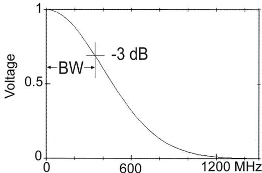
Figure 2: Frequency Response of 1 ns Risetime Gaussian
