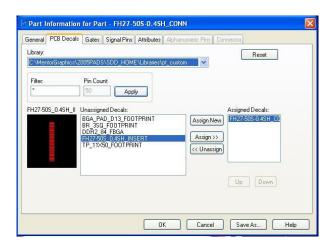
· Click "OK" on the "Part Information" window. Now this part is complete and can be added to PADS Logic and PADS Layout.
