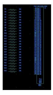
• Add the 75ohm, 0402 Resistors to the schematic
