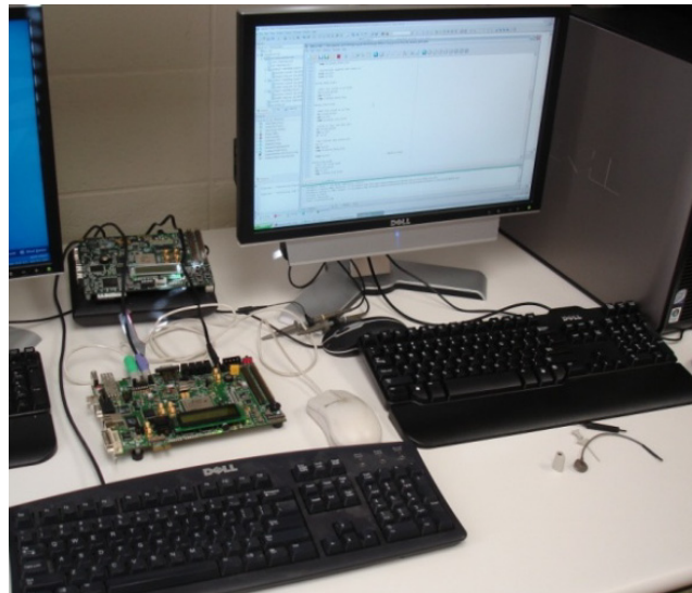
Fig. 1. Prototype system implemented on a Xilinx XUPV5 evaluation board.
