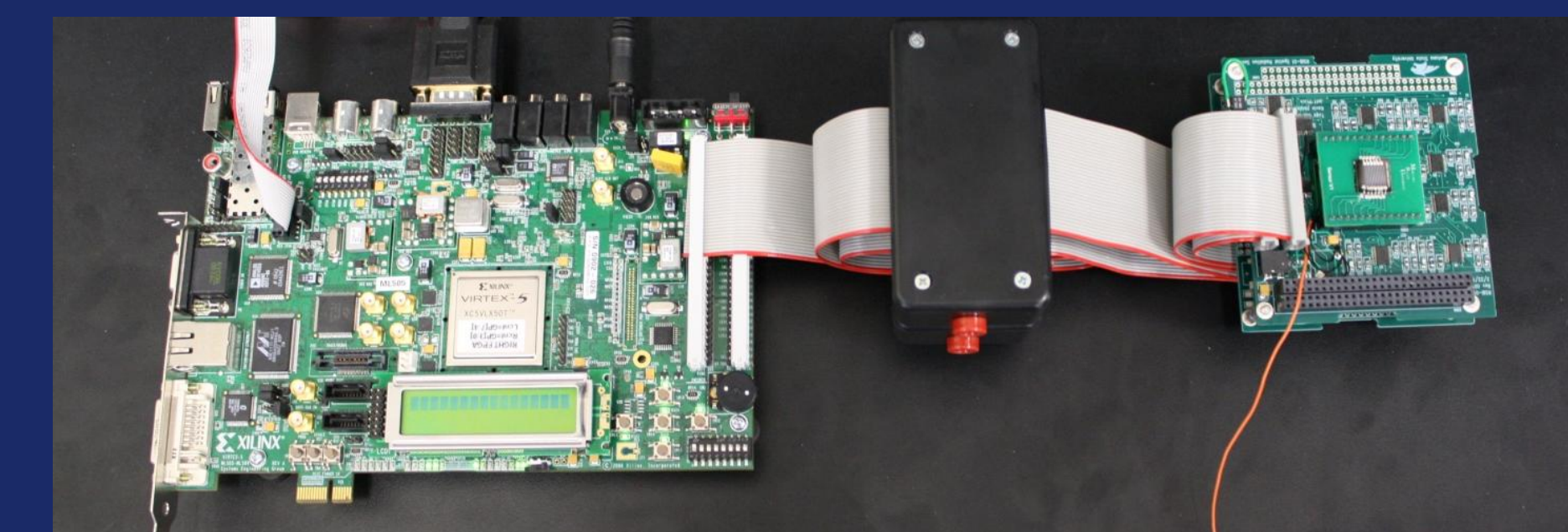
Fig 13. Entire System with FPGA (left), Sensor & Amp board (right) and clamping diode box (middle)
