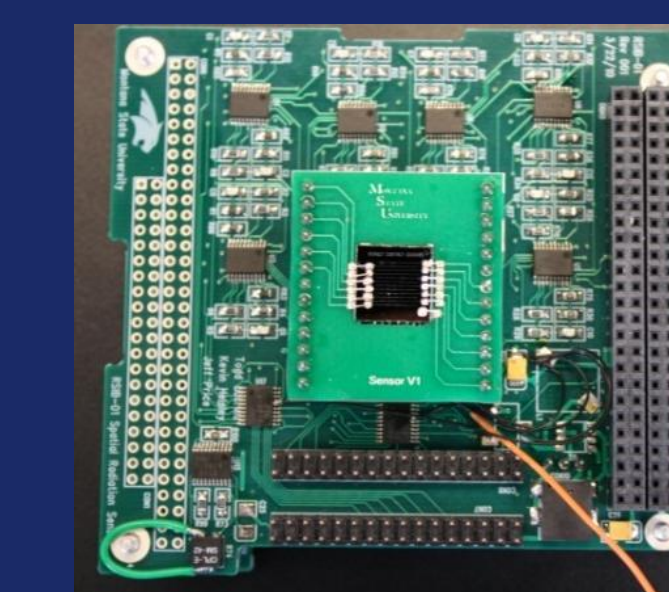
Fig 10. Amplifier Board containing 24 channels.
