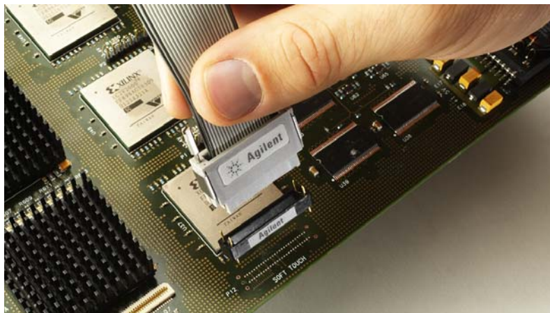
Figure 1. Physical Connection of a Connectorless Probing Technology
