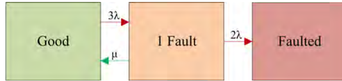
Figure 8.5: Markov State Transition Diagram - TMR System with scrubbing
