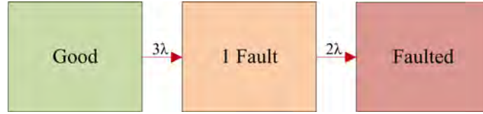
Figure 8.4: Markov State Transition Diagram - TMR System without scrubbing
