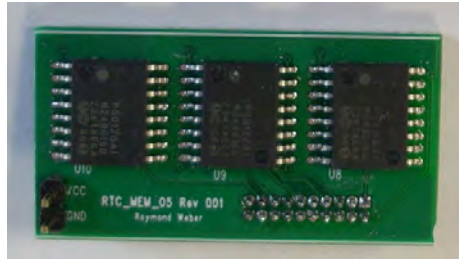
Figure 3.5: Phase Ram Daughtercard designed for the hardware stack.
