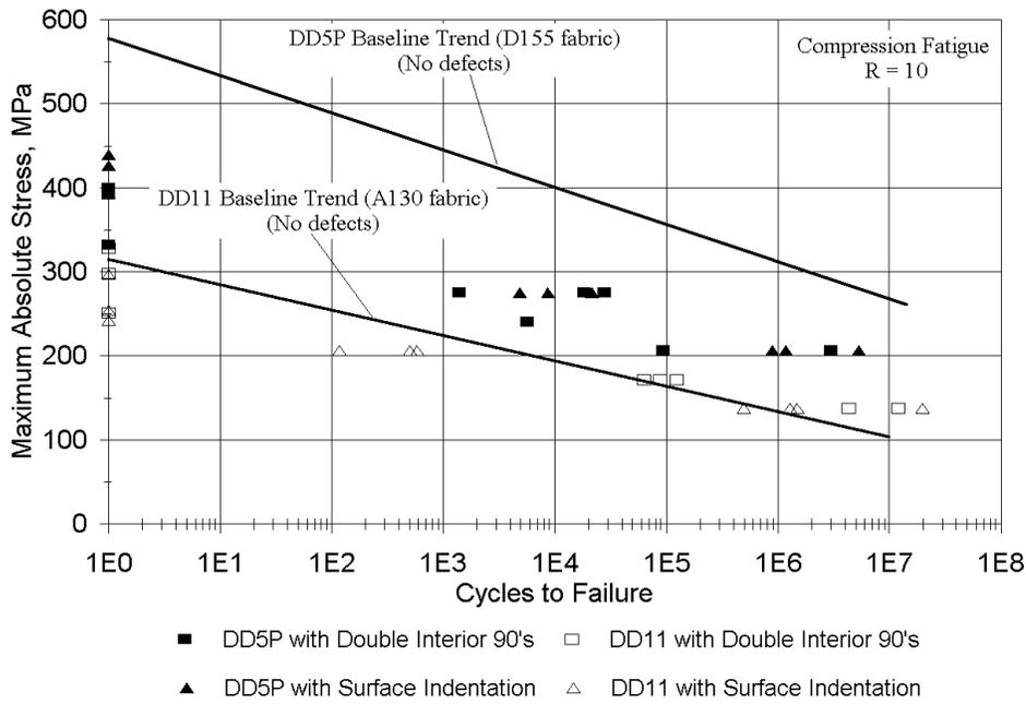
**Figure 6. Effects of Surface Indentation and Interior Inclusions on Compression Fatigue Resistance, R = 10.**
