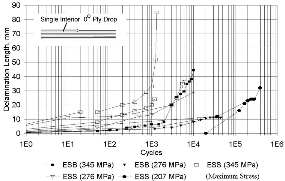
Figure 4. Typical Delamination Length vs. Cycle Data for Laminates ESB (D155 fabric) and ESS (A130 fabric) With a Single Interior Ply Drop.
