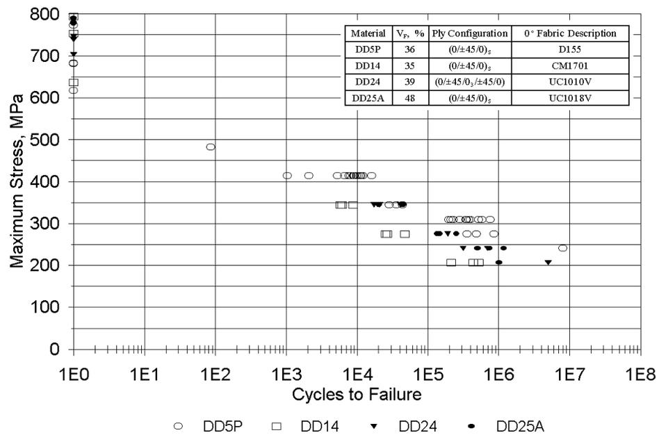
Figure 2. Tensile Fatigue Data Comparing Baseline Laminate (DD5P) With Laminates Based on Warp Unidirectional Fabrics, R = 0.1
