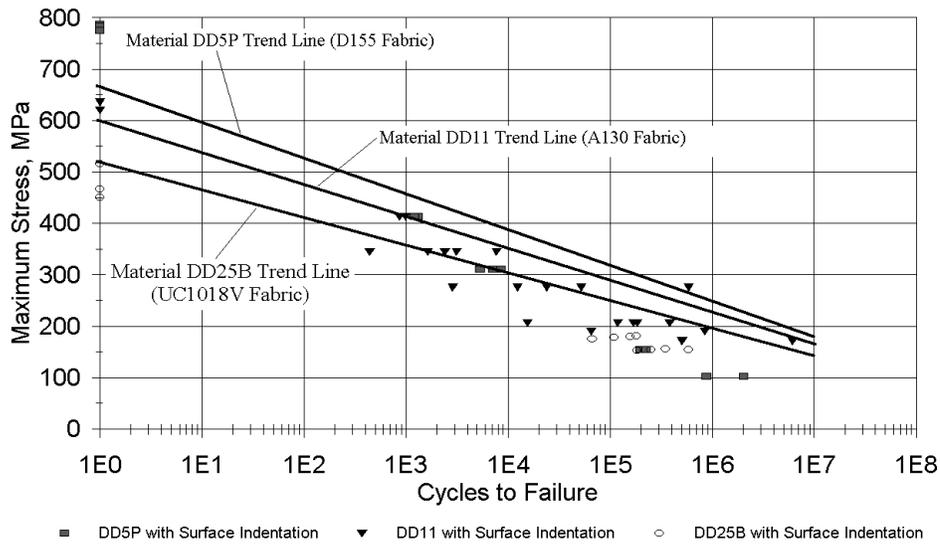
**Figure 7. Tensile Fatigue For Coupons Containing a Surface Indentation Compared With Trend Line For Base Laminates Without Indentations, R = 0.1 (See Figure 5).**
