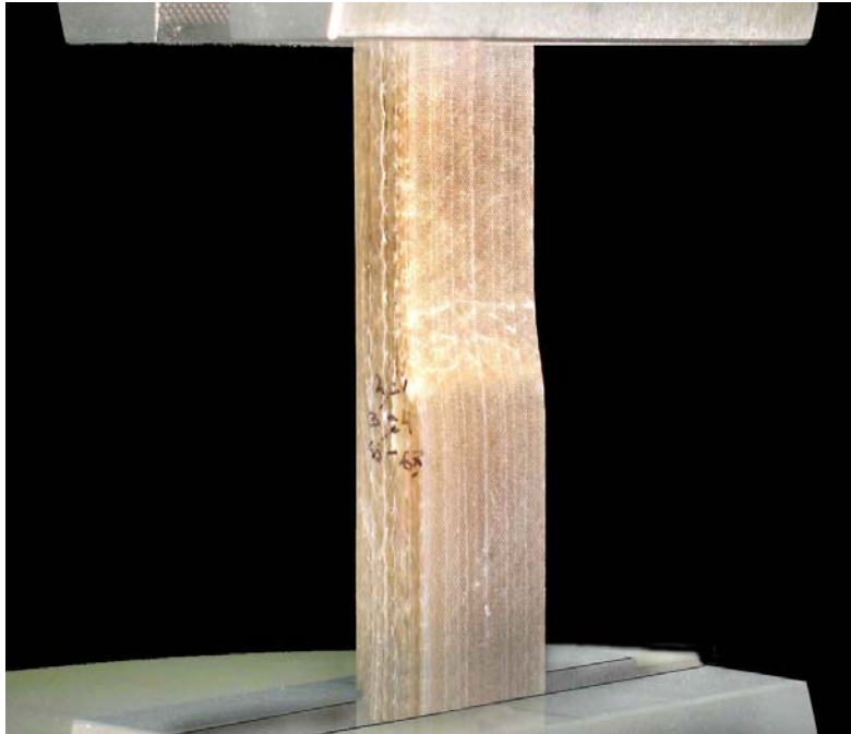
Figure 3. Complex Coupon with Fatigue Damage at Ply Drops, VE-2 Resin.
