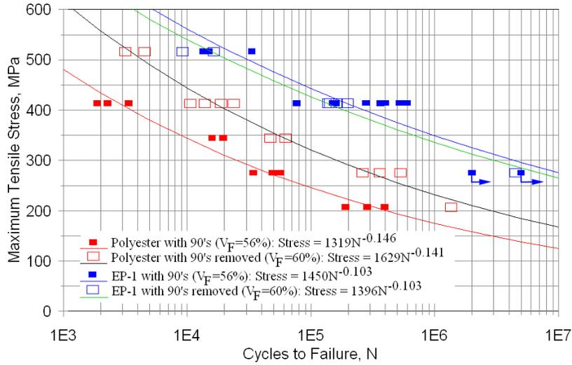
Figure 5. Effects of removing transverse backing strands on fabric data from Figure 4.
