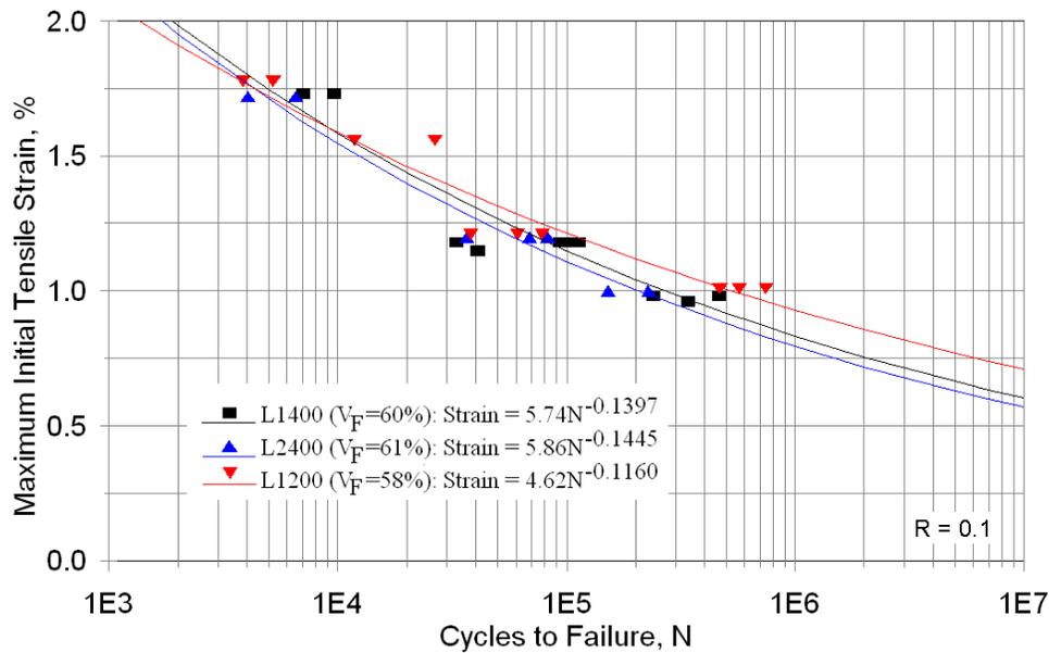
Figure 8. Stress (top) and strain (bottom) vs. cycles for MD laminates fabricated with three different weight UD fabrics from Table 6, epoxy EP5, R = 0.1.
