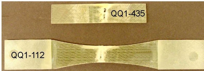
Figure 3. Failed Fatigue Specimens, Showing Grip-Edge Failure for a Rectangular Specimen (Top) and Gage Section Failure for a Dog-bone Specimen.
