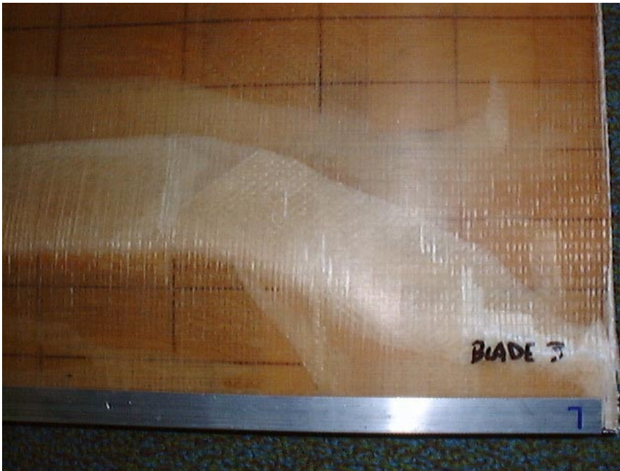
Figure 6-10. failures of the B-series panels tested in the SSSS condition
