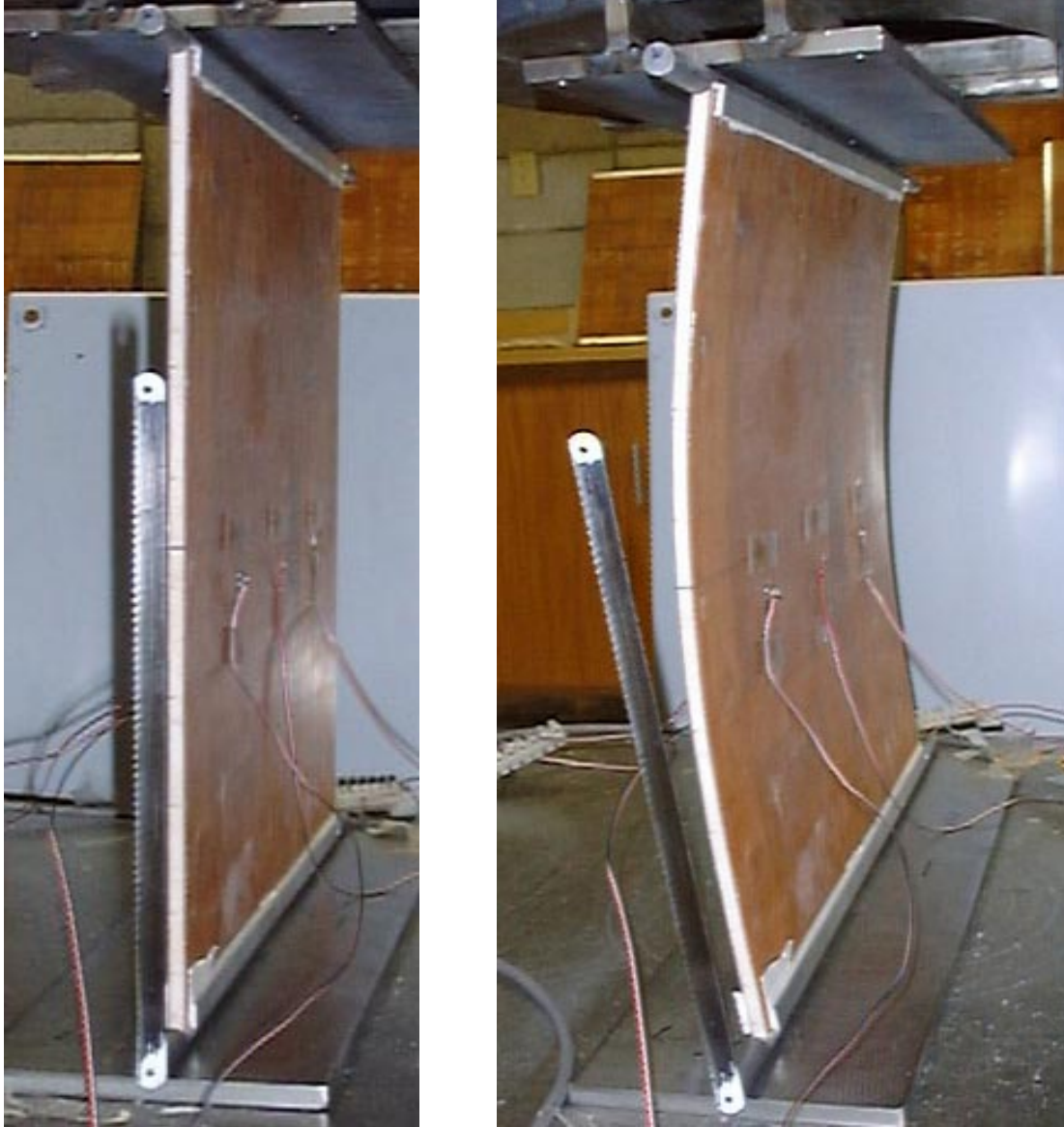
Figure 3-5. demonstration of the free rolling ability of the test fixture a). SFSF setup for roller rotation test b). roller rotation in the buckled configuration
