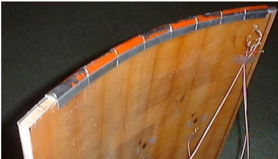
Figure 3-4. the curved test fixture attached to the panel, shown after testing
