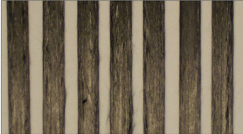
Figure 71: 60 min \text{HNO}_3 / 20 sec 1M NaOH treated rod surfaces before secondary epoxy infusion
