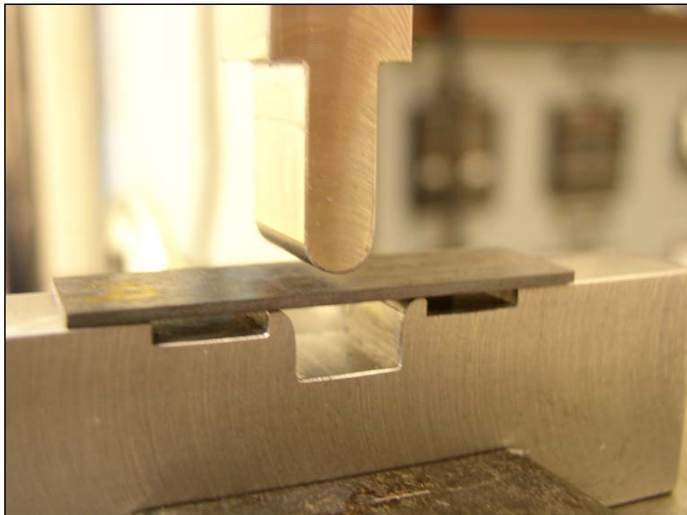
Figure 81: SBS coupon about to undergo loading
