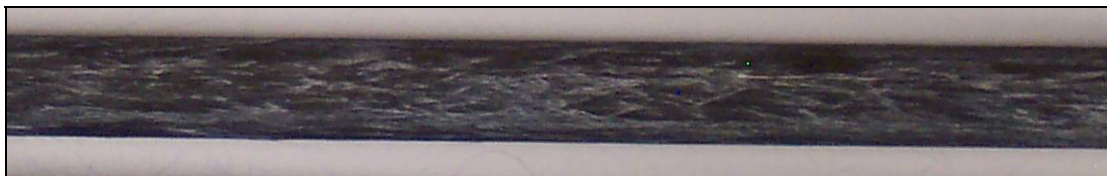
Figure 53: Surface of 60 min \text{HNO}_3 treated rod
