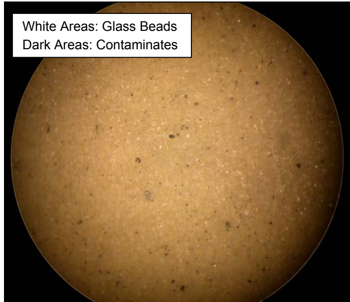
Figure 49: 16x magnification of glass bead media
