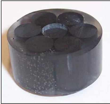
Figure 120: Typical pushout coupon interface failure appearance
