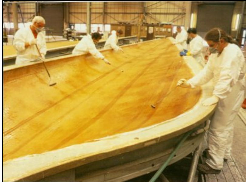
Figure 3: Physically laying up half a blade skin [5]
