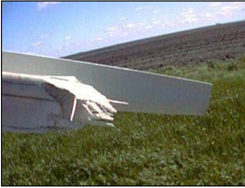
Figure 7: Damaged blade after tower strike compared to undamaged blade [12]
