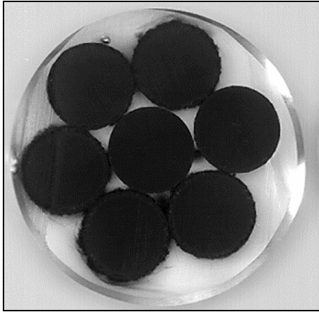
Figure 74: Washed 60 min \text{HNO}_3 rod pack profile
