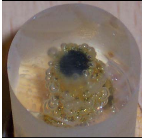
Figure 58: Unwashed 60 min HNO 3 single rod trial
