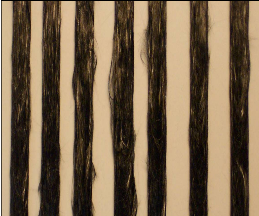
Figure 73: 60 min \text{HNO}_3 / 20 sec 5M NaOH treated rod surfaces before secondary epoxy infusion
