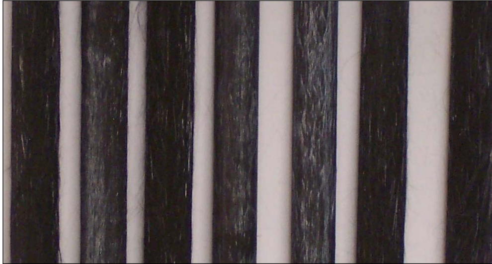
Figure 70: 60 min HNO 3 treated rod surfaces before secondary epoxy infusion
