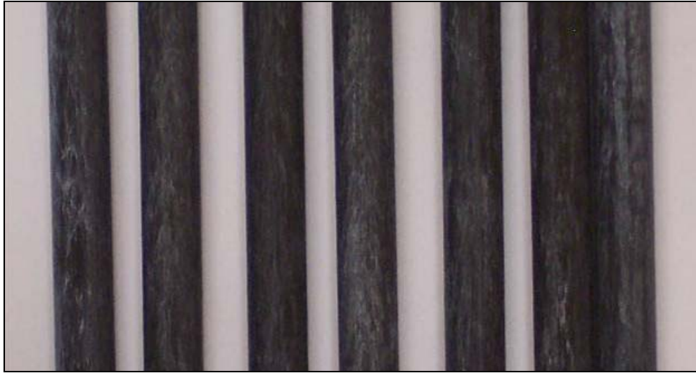
Figure 68: 15 min HNO 3 treated rod surfaces before secondary epoxy infusion
