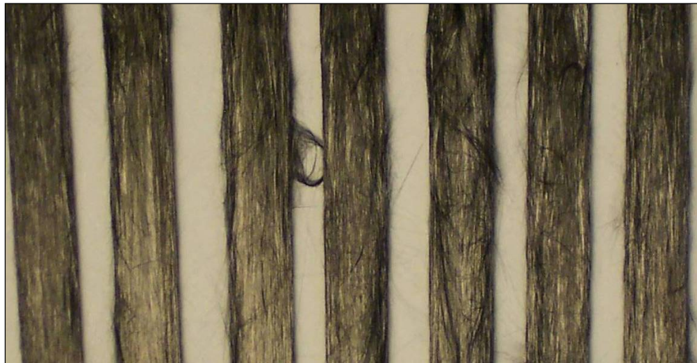
Figure 72: 60 min \text{HNO}_3 / 20 sec 2M NaOH treated rod surfaces before secondary epoxy infusion
