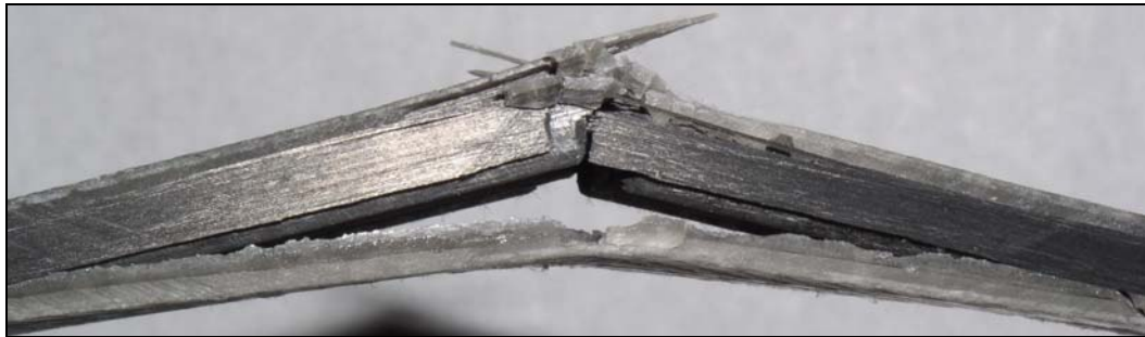
Figure 36: Three-point bending test result showing that the secondary resin had peeled off the pultrusion
