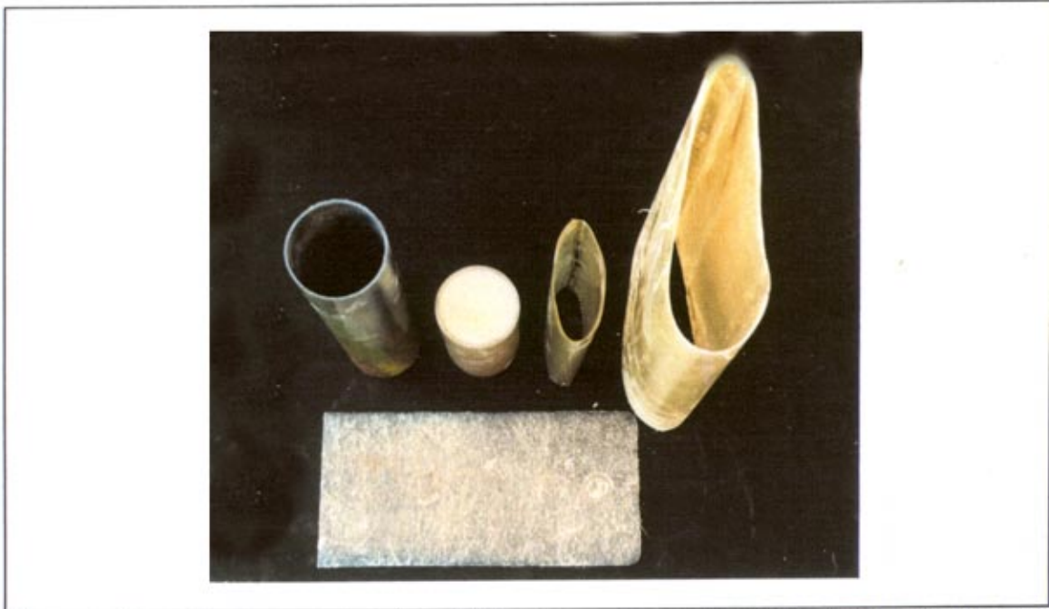
Figure 7. Photograph of moldings made using the RTM equipment developed in this study.
