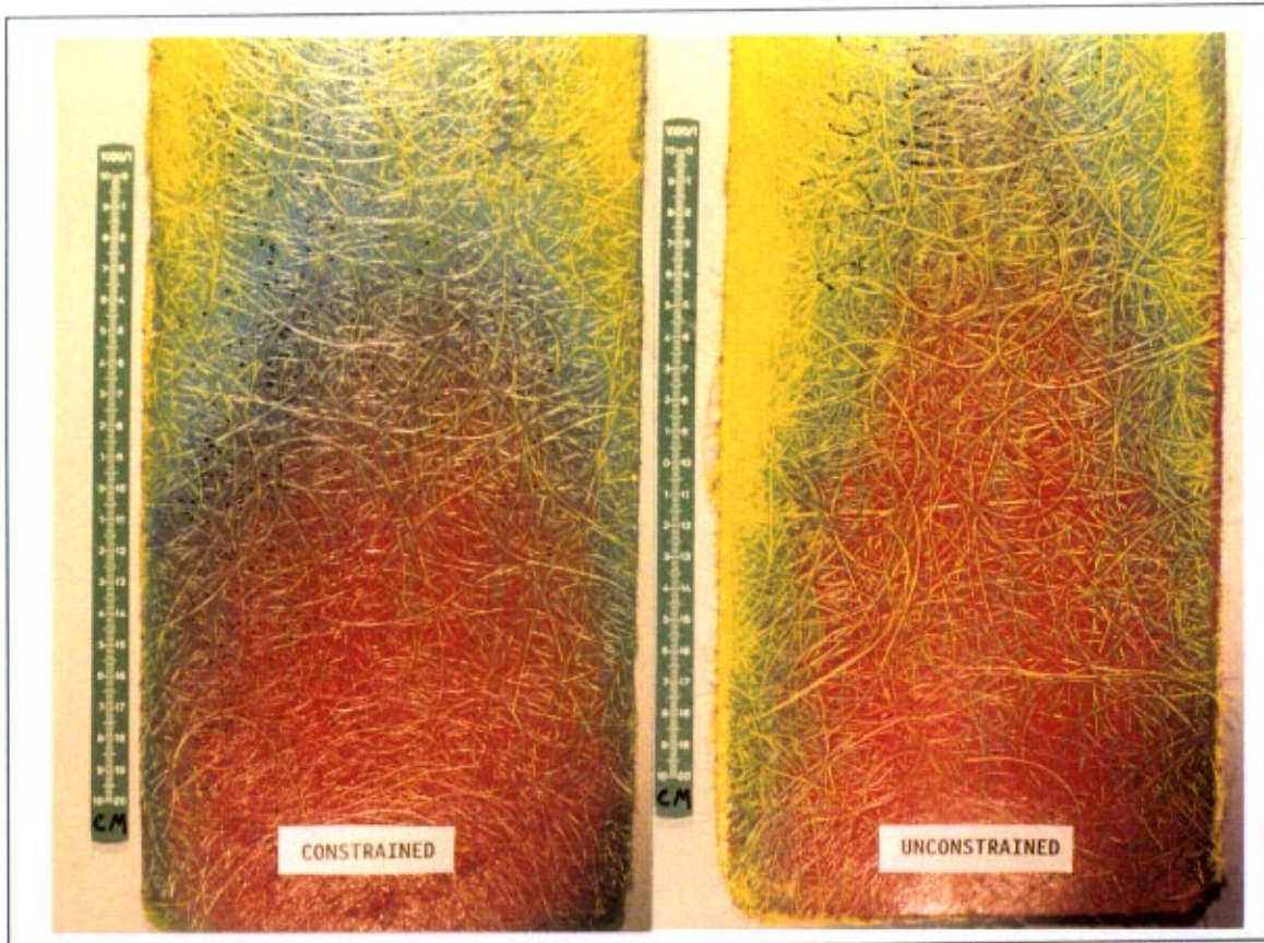
Figure 24. Photographs of cured parts molded with and without stiffeners.
