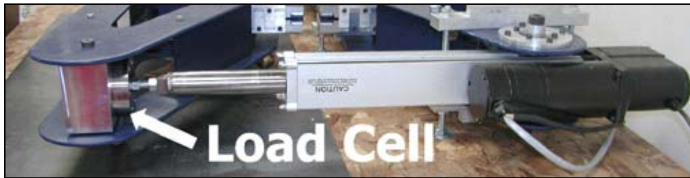
Figure 15. Actuator, load cell, and pivot block on the IPL [7]
