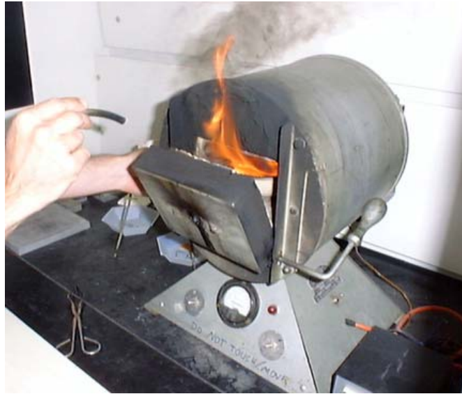
Figure 10: Burn-off test showing combustion products.
