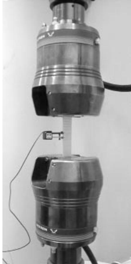
Figure 29. Flat specimen testing with extensometer.
