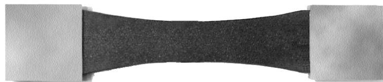
Figure 3.5. Unnotched tension sample.
