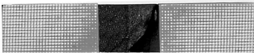
Figure 3.7. Unnotched compression sample.
