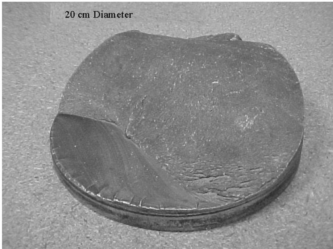
Figure 8. Hydro-Turbine Shaft Failure
