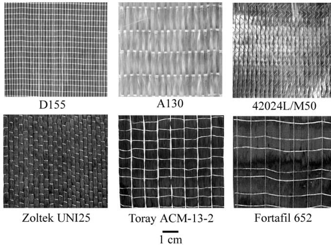
Figure 1. Glass (top) and Carbon Fabrics Used in This Study.
