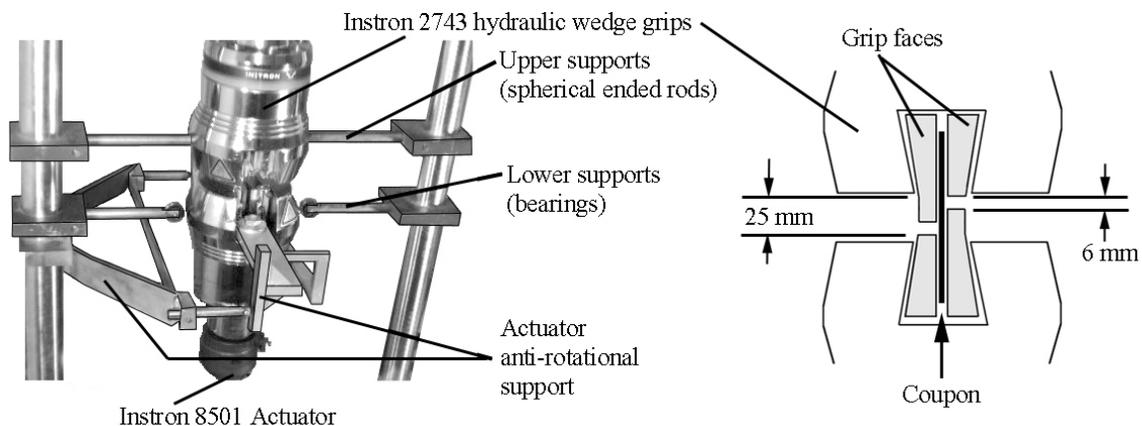
Figure 4. Actuator Lateral and Rotational Constraints for Compression Tests (left) and Coupon Wedge Grips (Right).
