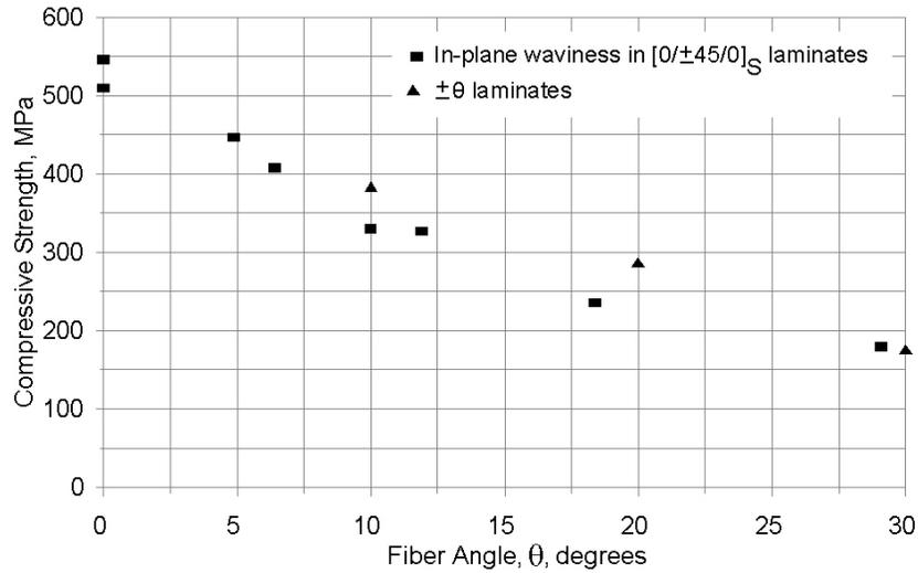
Figure 13. Compressive Strength With Waviness in all  $0^\circ$  Plies versus Maximum Misalignment Angle ( $\theta$ ), Compared with Data from  $\pm\theta$  Off-Axis Laminates [4].
