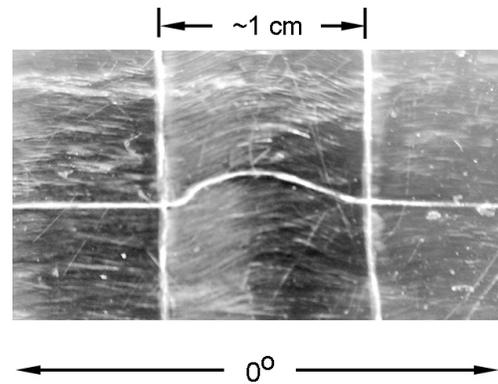
Figure 2. In-Plane Waviness in a Single-Ply Laminate of Fortafil 652 Carbon Fiber/Epoxy Processed by RTM [4].
