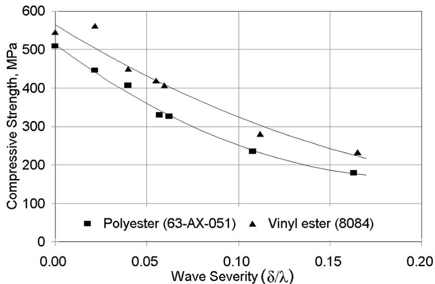
Figure 12. Effects of Resin Matrix Toughness on Compressive Strength of Laminates Containing Various Severities of Waviness (waviness in all  $0^\circ$  plies) [4].
