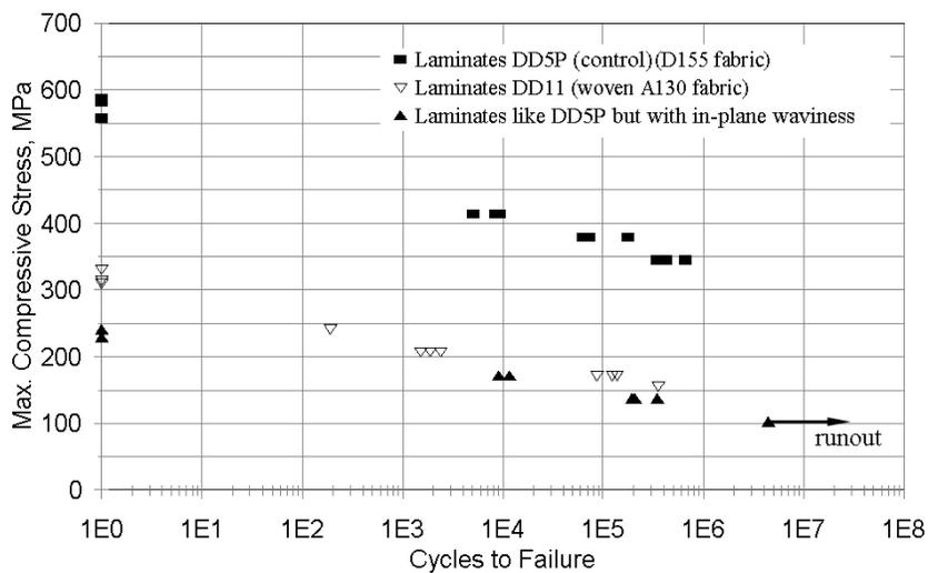
Figure 15. Compressive Fatigue Properties for Laminates with Four Layer In-Plane (4 mm/35mm) Waviness and Through-Thickness (DD11) Waviness Compared With Control Laminate DD5P,  $R = 10$  [4].
