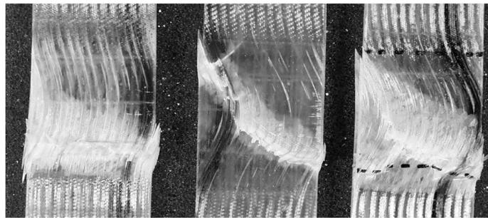
Figure 14. Static Compression Failures and Fatigue Compression Failures (left: static/ vinyl ester resin; center: static/ polyester resin; right: fatigue/ polyester resin) [4].
