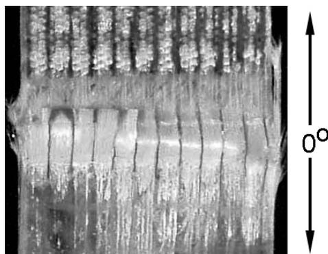
Figure 5. Static Compression Failure Mode for a Typical  $[0/\pm 45/0]_S$  Laminate Containing D155 Unidirectional Fabric for the  $0^\circ$  Plies (Figure 1).
