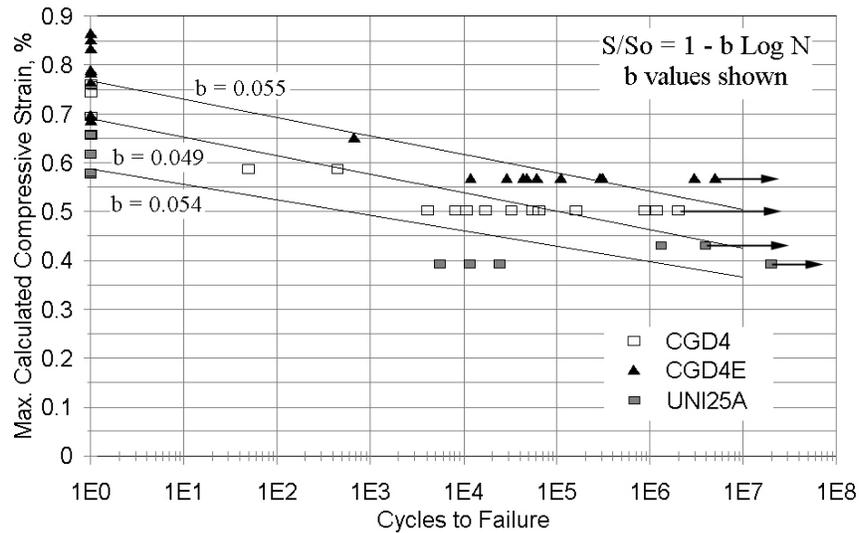
Figure 6. Compression Fatigue Data for Carbon Fiber and Hybrid Laminates: CGD4 and CGD4E, ( $\pm 45/0_3/\mp 45$ ),  $0^\circ$ : Toray Stitched Carbon Fabric ACM-13-2,  $\pm 45$ : DB120 Glass; UNI25A, Unidirectional  $[0_3]$ , Zoltek UNI25 Woven Carbon Fabric. Resins are Derakane 8084 Vinyl Ester for CGD4 and UNI25A, and Prime 20 Epoxy for CGD4E.
