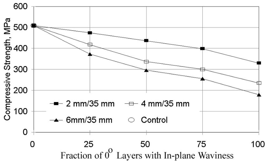
Figure 11. Effects of Multi-layer In-plane Waviness on Compressive Strength for various wave parameters  $\delta/\lambda$ .
