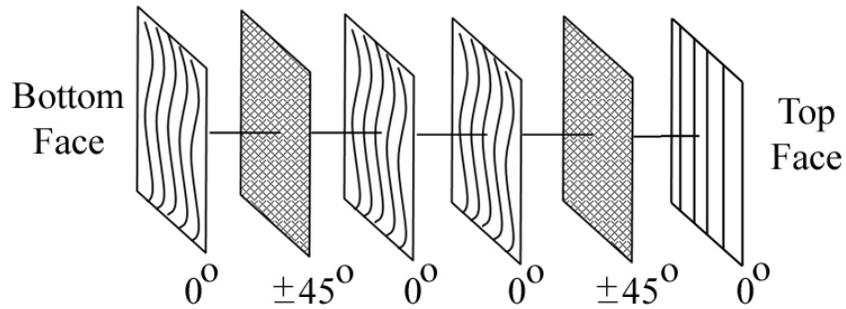
Figure 10. Laminate Configuration with Three Layers of In-Plane Waviness.
