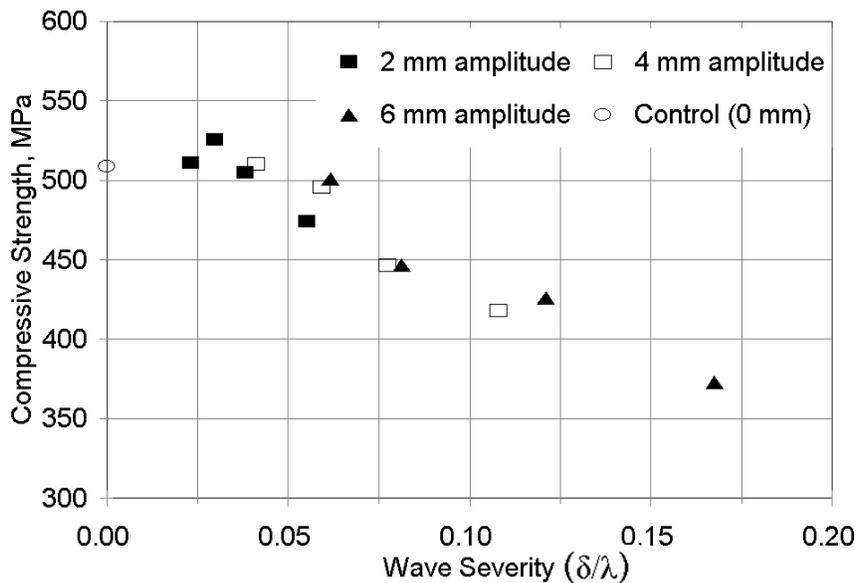
Figure 9. Effects of Wave Severity on Compressive Strength; Waviness in a Single Surface Ply of a  $[0/\pm 45/0]_S$  Laminate.
