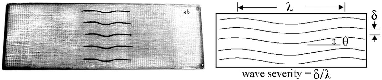
Figure 3. Laminate with Introduced Waviness (left) and Waviness Characterization (Right) [4].
