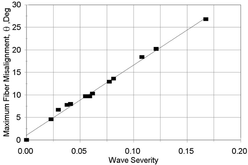
Figure 8. Correlation between Wave Severity and Maximum Angle of Fiber Misalignment,  $\theta$ .
