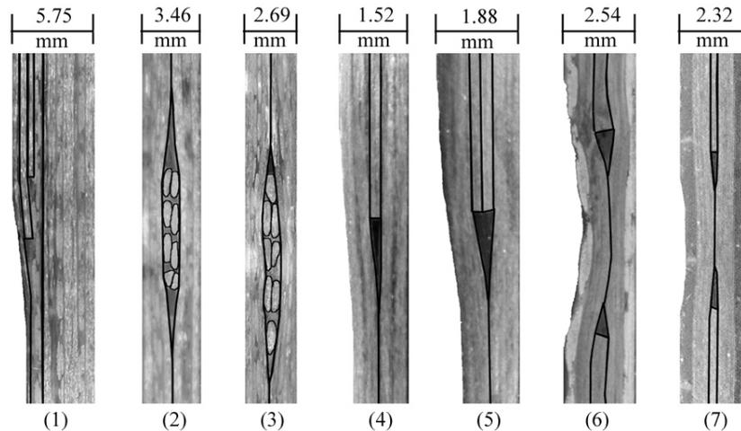
Figure 7. Enhanced Cross-Sectional Views of Materials Containing Ply Drops, Joints and Inclusions (See Table 2 for details).
