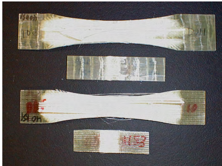
FIGURE 32 (j) Standard structural material at low fiber content, 72% 0's. From top to bottom; Material DD11 (A130 fabric 0's, V_F = 31\% ); tensile fatigue ( R = 0.1 , 276 MPa); compression fatigue ( R = 10 , 172 MPa); and Material DD6 (D155 fabric 0's, V_F = 31\% ); tensile fatigue ( R = 0.1 , 276 MPa); and compression fatigue ( R = 10 , 379 MPa).
