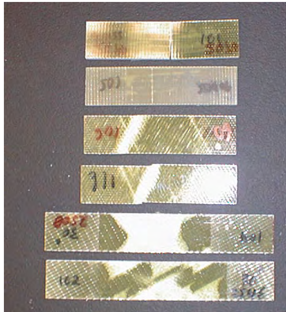
FIGURE 32 (n) D155 fabric, angled composites in static tension and tension fatigue ( V_F = 38 to 40\% ) from top to bottom: \pm 90^\circ tensile fatigue ( R = 0.1 , 17.2 MPa); and static tension; \pm 60^\circ , static tension and tension fatigue ( R = 0.1 , 19 MPa); \pm 30^\circ static tension and tension fatigue ( R = 0.1 , 121 MPa).
