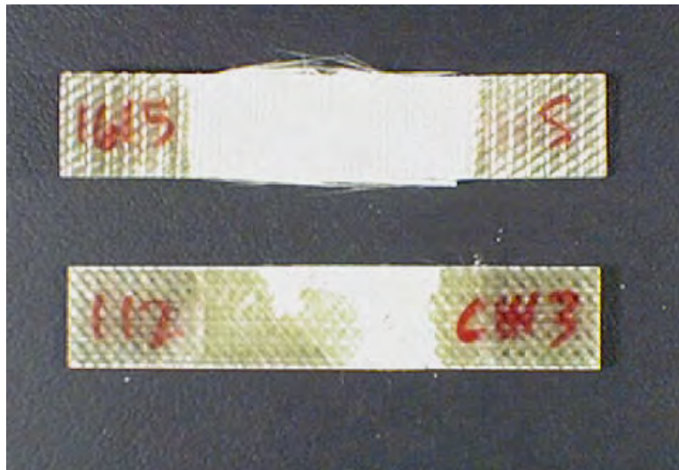
FIGURE 32 (h) High fiber content, low percent 0's. Material CH13 ( V_F = 48\% , 24% 0's). Static tensile coupon (top) and tensile fatigue ( R = 0.1 , 172 MPa).
