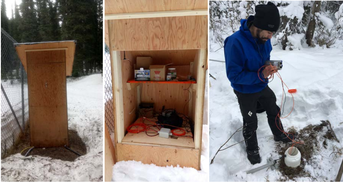
Figure 2: Left and Center: Central element of the infrasound station enclosed within the wooden structure with power supply, data storage and data transmission units as well as one infrasound sensor. Right: One of the outer sensors being installed, showing the transducer inside a partially buried plastic housing. Left and center photos by Lisa Dreier (May 11, 2017 and March 17, 2017). Right by Chris Argue, DAC (12 December, 2016).
