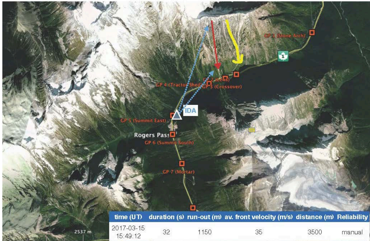
Figure 10: Example output from the infrasound system showing the back-azimuth (upper dashed blue arrow), the signal migration (lower dashed blue arrow) and inferred flow of the detected avalanche (red arrow). The observed event is shown with the yellow line. The incorrect attribution is likely due to topographic shielding.
