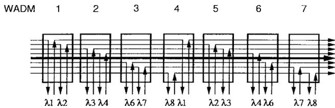
Fig. 4. Simulation add-drop scheme indicating the exact WADM where each channel pair is dropped and then added. Channels correspond to frequencies from 192.100 THz (for channel 8) to 193.500 THz (for channel 1) in 200-GHz steps. The add-drop scheme is periodically repeated after every seven WADM's.
