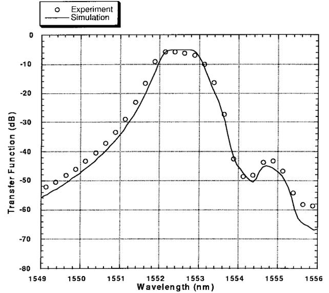
Fig. 3. Transmittance of MONET wavelength 3 through a MUX. As explained in [6], a MUX is a cascade of eight MI filters. ASE noise is inserted on input 3 (associated with wavelength 3) of the multiplexer and what is shown is the MUX output. We focus on transmittance at one wavelength.
