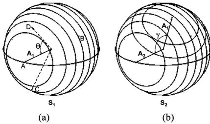
Fig. 4. (a) Isopenalty regions for one SOA and one fiber span; (b) polarization evolution (in this case rotation of the sphere) as signal goes through fiber and subsequent SOAs creates superimposed isopenalty regions.
