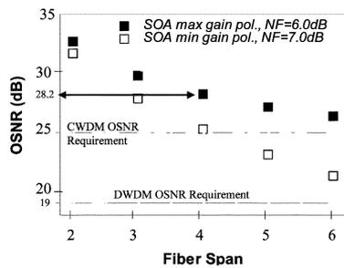
Fig. 2. Simulation results for OSNR after transmission versus fiber span in the case of SOA PDG of 1 dB and noise figure of 6.0 (maximum gain polarization) and 7.0 dB (minimum gain polarization). Polarization aligned to the maximum (minimum) amplifier gain axis is shown by solid (open) symbols. In general, for  $n$  fiber spans, there are  $n - 1$  SOAs in the cascade. Channel input power to each SOA stage for maximum gain polarization is  $-19.3$  dBm.
