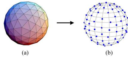
Fig. 3. (a) Tessellating the Poincaré sphere creates nonoverlapping triangular grids; (b) mapping the grid nodes to azimuth and ellipticity produces the uniformly distributed input polarization states used in the model.
