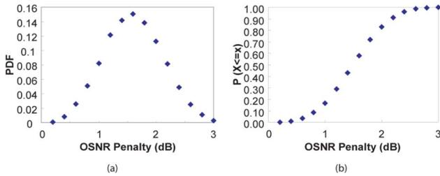
Fig. 5. (a) Polarization-induced OSNR-penalty pdf for the case of three SOAs or 320 km of path reach; (b) OSNR-penalty cdf for the same case.
