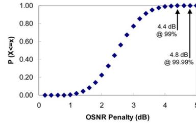
Fig. 6. Polarization-induced OSNR-penalty cdf for the case of five SOAs or 480 km of path reach.
