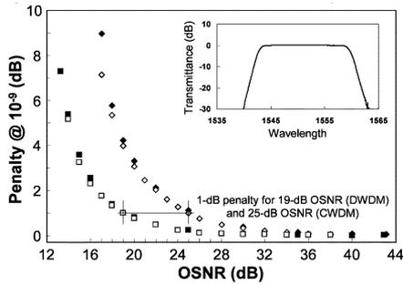
Fig. 1. APD receiver characterization for a CWDM channel (solid diamonds) and a DWDM channel (solid squares) at 2.5 Gb/s. The CWDM configuration uses a CWDM demultiplexer with 17-nm 3-dB bandwidth (inset). The DWDM configuration uses an optical filter with 0.25-nm 3-dB bandwidth. Simulation results (open symbols) closely match the experiment.
