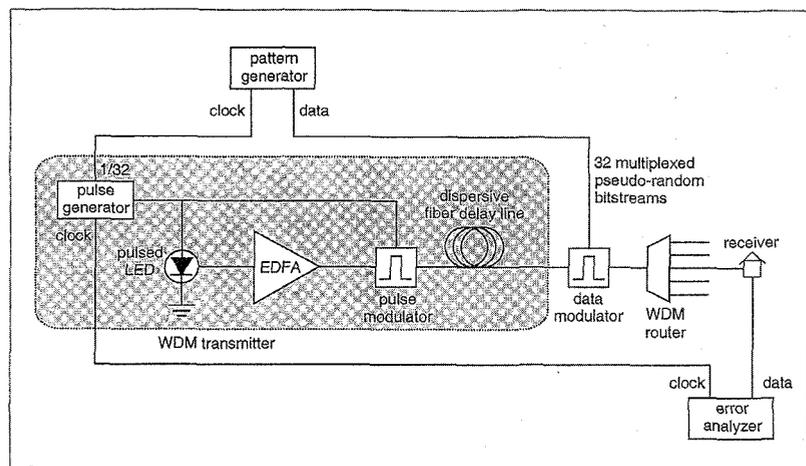
**CFI4 Fig. 1** Schematic of chirped WDM transmission system. Light from a pulsed LED transmitter is encoded at modulator with 32 multiplexed pseudorandom bitstreams. Wavelength channels are demultiplexed at an optical bandpass filter or WDM router, with individual bitstreams received and analyzed for errors.
