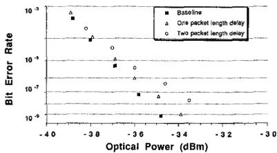
CFI2 Fig. 3 BER versus received optical power of the active WDM fiber loop buffer.
