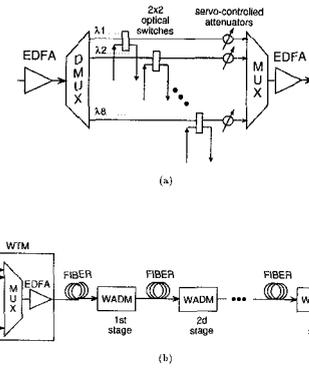
CFI3 Fig. 1 (a) Block diagram of a wavelength add-drop multiplexer (WADM); (b) block diagram of a cascade of WADMs.
