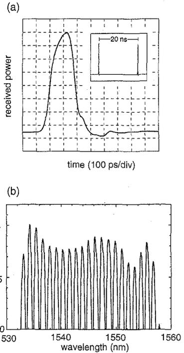
**CFI4 Fig. 2** WDM transmitter optical power in 0.05 nm bandwidth (a) after power-splitting tap, showing 200 ps pulses at 50 Mb/s bitrate. Inset shows full 20-ns bit period. Spectrum (b) after data-encoding modulator, driven by an RZ pattern with all channels on, showing 20 signal channels, spaced at 1.2 nm.
