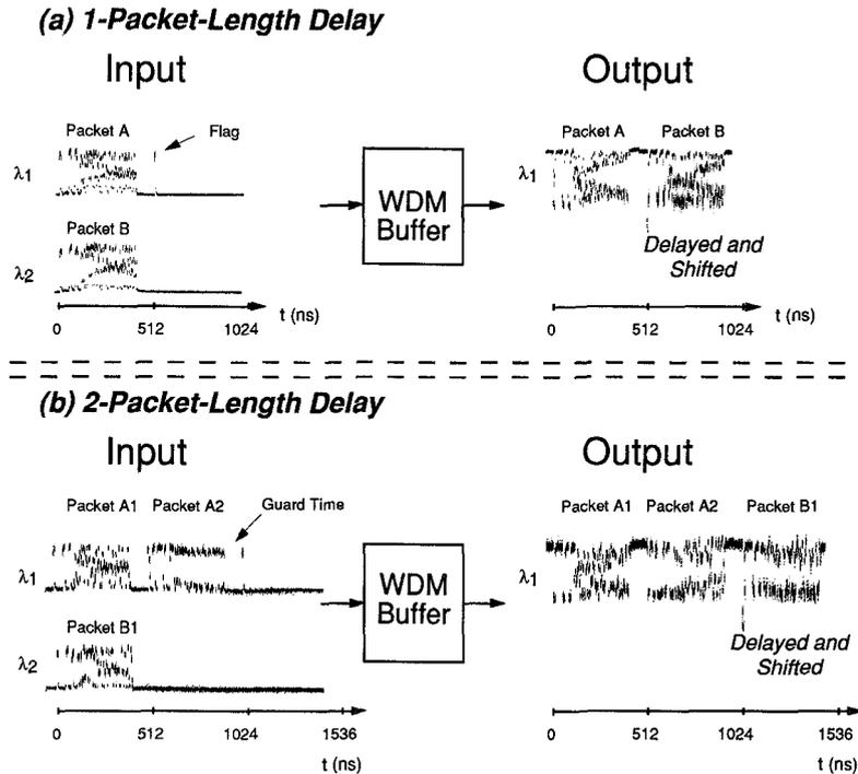
CFI2 Fig. 2 (a) Oscilloscope trace of the inputs ( $\lambda_1$  and  $\lambda_2$ ) and output ( $\lambda_1$ ) for one-packet-length delay. (b) Oscilloscope trace of the inputs ( $\lambda_1$  and  $\lambda_2$ ) and output ( $\lambda_1$ ) for two-packet-length delay.
