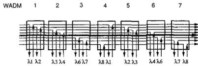
**CFI3 Fig. 2** Simulation add-drop scheme indicating the exact WADM where each channel pair is dropped and then added. Channels correspond to frequencies from 192.100 THz (for channel 8) to 193.500 THz (for channel 1) in 200 GHz steps. The add-drop scheme is periodically repeated after every seven WADMs.
