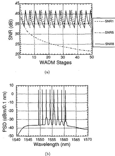
**CFI3 Fig. 3** (a) Optical signal-to-noise ratio (SNR) in 0.1 nm resolution bandwidth as a function of the number of WADMs traversed. SNR varies between 34 dB at the drop site and 42 dB just after addition for all wavelengths except  $\lambda_5$  whose SNR drops to 21.8 dB; (b) Power spectral density (PSD) in dBm/0.1 nm after the 50 WADM cascade.
