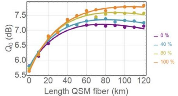
Fig. 3. Optimum Q-factor  $Q_0$  as a function of the QSM fiber length per span for different MPI compensation levels.
