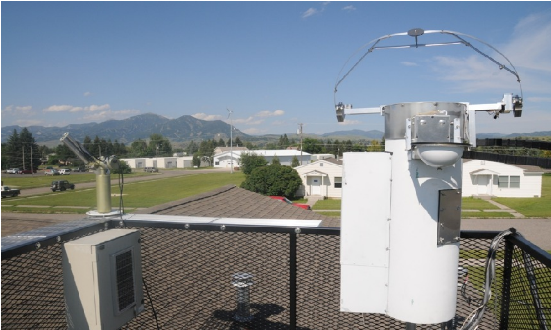
Figure 1. Photograph of the Montana State University all-sky polarization imager (right) and solar radiometer (left).
