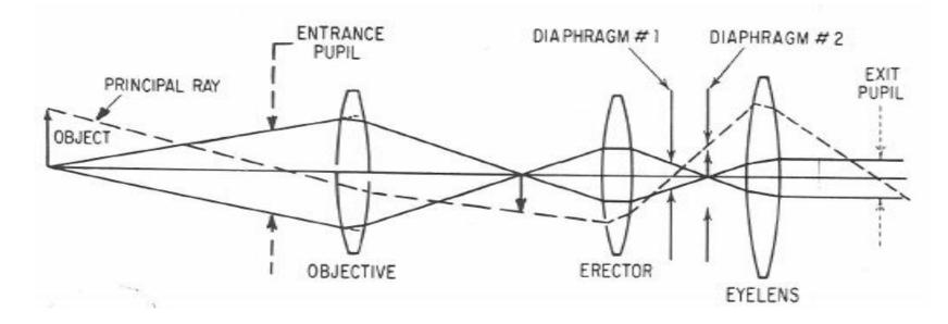
Sfc 1:  $f_1 = 10 \dots D_1 = 2.3 \dots t_1 = 16.5$ Sfc 2:  $f_2 = 2 \dots D_2 = 1.7 \dots t_2 = 2.38$ Sfc 3:  $\varphi_3 = 0 \dots D_3 = 0.25 \dots t_3 = 1.62$
