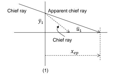
From the triangle in the figure  $\dots \bar{u}_1 = \frac{-y_1}{x_{ep}}$ (the minus sign is from the sign convention, as the diagram is drawn for a negative angle)
