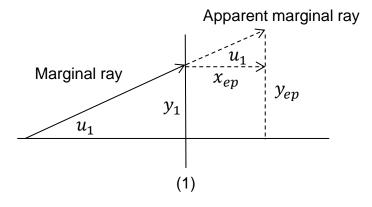
From the triangle in the figure ...  $u_1 = \frac{y_{ep} - y_1}{x_{ep}}$
