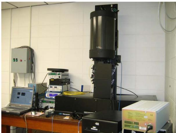
Fig. 8. A picture of the DIAL instrument in its operational form inside the rooftop room of Cobleigh Hall at Montana State University.
