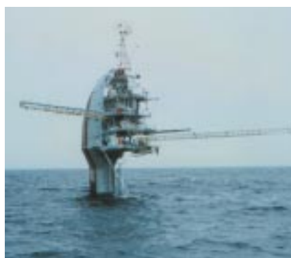
Figure 2. The Floating Instrument Platform (FLIP, operated by Scripps Institution of Oceanography), where NOAA deployed laser-glint sensors in September 1995 for measuring ocean surface roughness.
