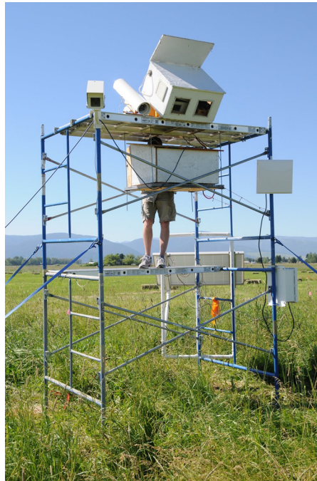
Fig. 1 Scaffold used to mount the thermal IR imager (in the white tube) and a visible-near-infrared multispectral imager (in the white box with the open back).
