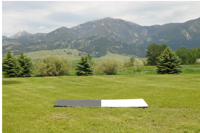
Fig. 7 Photograph of a plywood black-and-white reflectance calibration panel, which is laid on the ground within the imager's field of view to provide a reflectance calibration. Later versions were painted on canvas tarps.
