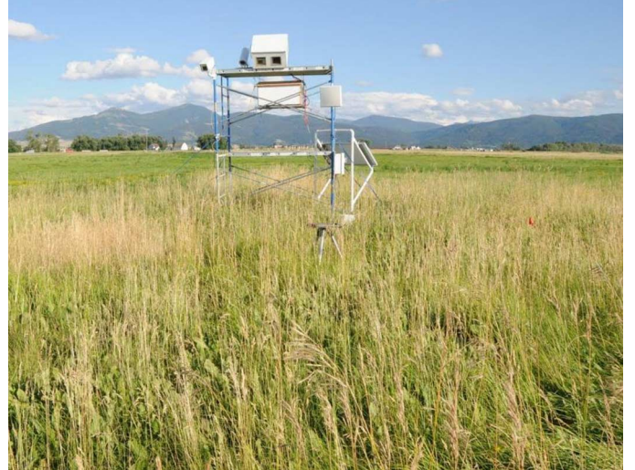
Fig. 1. Side-by-side Vis/NIR and LWIR imagers mounted on a scaffold to measure vegetation reflectance and emission, respectively, at the ZERT field in Bozeman, Montana. The tripod in front of the scaffold is a mount that holds a reflectance panel to calibrate the Vis/NIR images.
