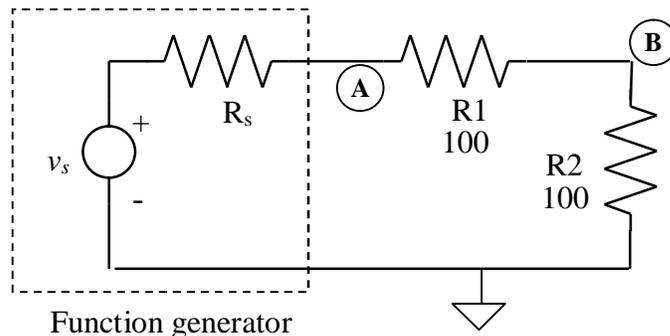
9. Connect the oscilloscope ground clip to the grounded node in the circuit. Measure the voltage amplitude using the MEASURE feature at nodes **A** and **B**. Set the timebase to display at least two periods of the waveform for these measurements. Experiment with the timebase setting until less than one period is displayed. Does the measured V<sub>pp</sub> change? Return the timebase setting to have multiple periods displayed.
