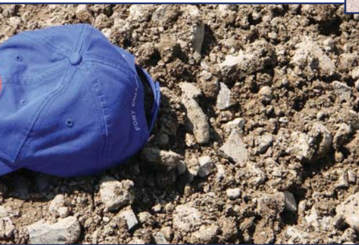
Above: Ripped Roadway Gravel Crushed
