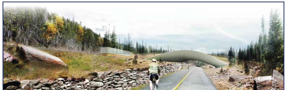
The Zwarts & Jansma Architects (Amsterdam) proposed “‘curves’ as the main organizing elements for the architecture of the load-bearing structure itself. In cross section the curve ‘contains’ the landscape and the wildlife that overpasses. At the same time it is an ‘inviting’ shape in the perpendicular direction for the traffic that underpasses.”
