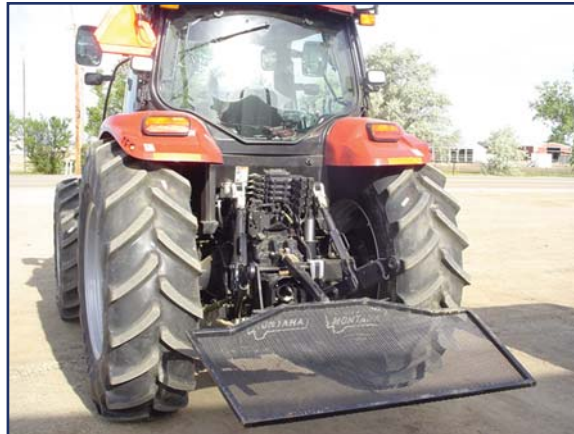
Guard Dropped Down for Cleaning
