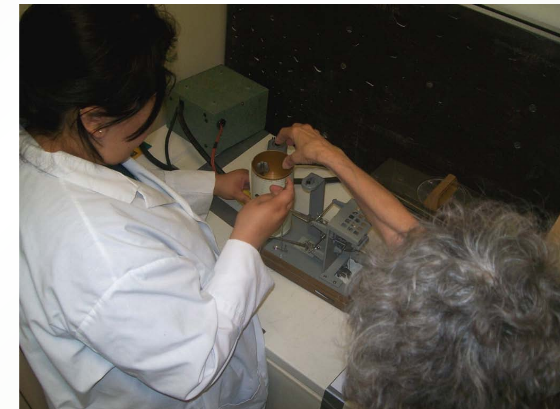
Figure 7. Changing the record chart for the 7-day, continuous recording thermo-hydrograph in the environmental chamber where both mass cultures of bruchid beetles are kept and the bioassays are conducted.
