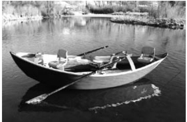
The 300 lb. Kingfisher model driftboat has a honeycomb Kevlar-reinforced bottom panel, mahogany and fiberglass reinforced side panels, and nearly 10 cu. ft. of dry storage space. Photo courtesy of Montana Boatbuilders
