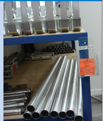
Orange kanbans from in-house parts area go to collection box to trigger builds when inventory levels drop to a fixed point.
