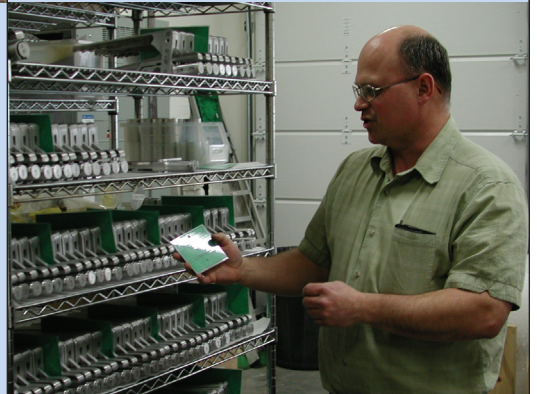
Bryan Osborne holds green Kanban used at intervals in finished goods to trigger another order to the factory floor, as tools are shipped.
