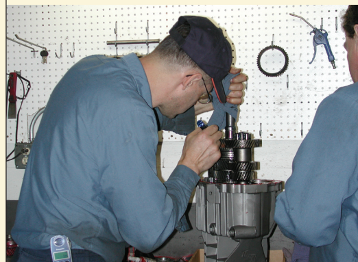
Richard double checks a difficult fitting in a transmission re-build.
