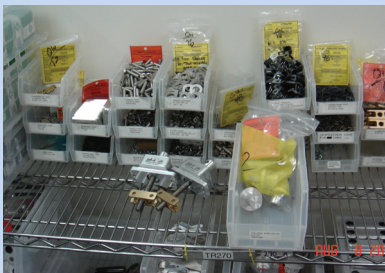
Yellow and orange kanbans trigger replenishment actions for parts.
