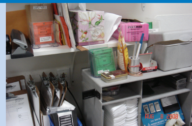
Shipping work station has a collection box for kanbans that enable production manager to schedule the shop by placing them on the FIFO board as orders go out.
