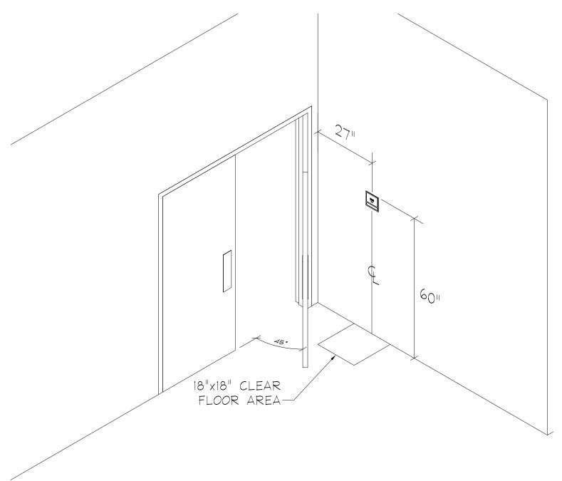
NOTE: WHERE THERE IS NO WALL SPACE ON THE RIGHT SIDE OF DOUBLE DOORS, SIGN WILL BE MOUNTED ON THE NEAREST ADJACENT WALL. SIGNS SHALL BE LOCATED SO THAT A CLEAR FLOOR AREA 18" MIN. BY 18" MIN. CENTERED ON THE TACTILE TEXT IS PROVIDED BEYOND THE ARC OF ANY DOOR SWING BETWEEN THE CLOSED POSITION AND 45 DEGREE OPEN POSITION.
