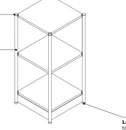
**Leveling guides** adjust for installations on uneven floors. Adjustability range is 17/8".
