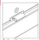
**Optional locks on doors** are located centered on the door panel and directly above the door pull.
