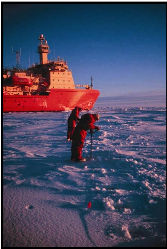
Drilling holes to measure the thickness of a first-year sea ice floe in the Ross Sea, August 1995, R.V. Nathaniel B. Palmer in the background.
