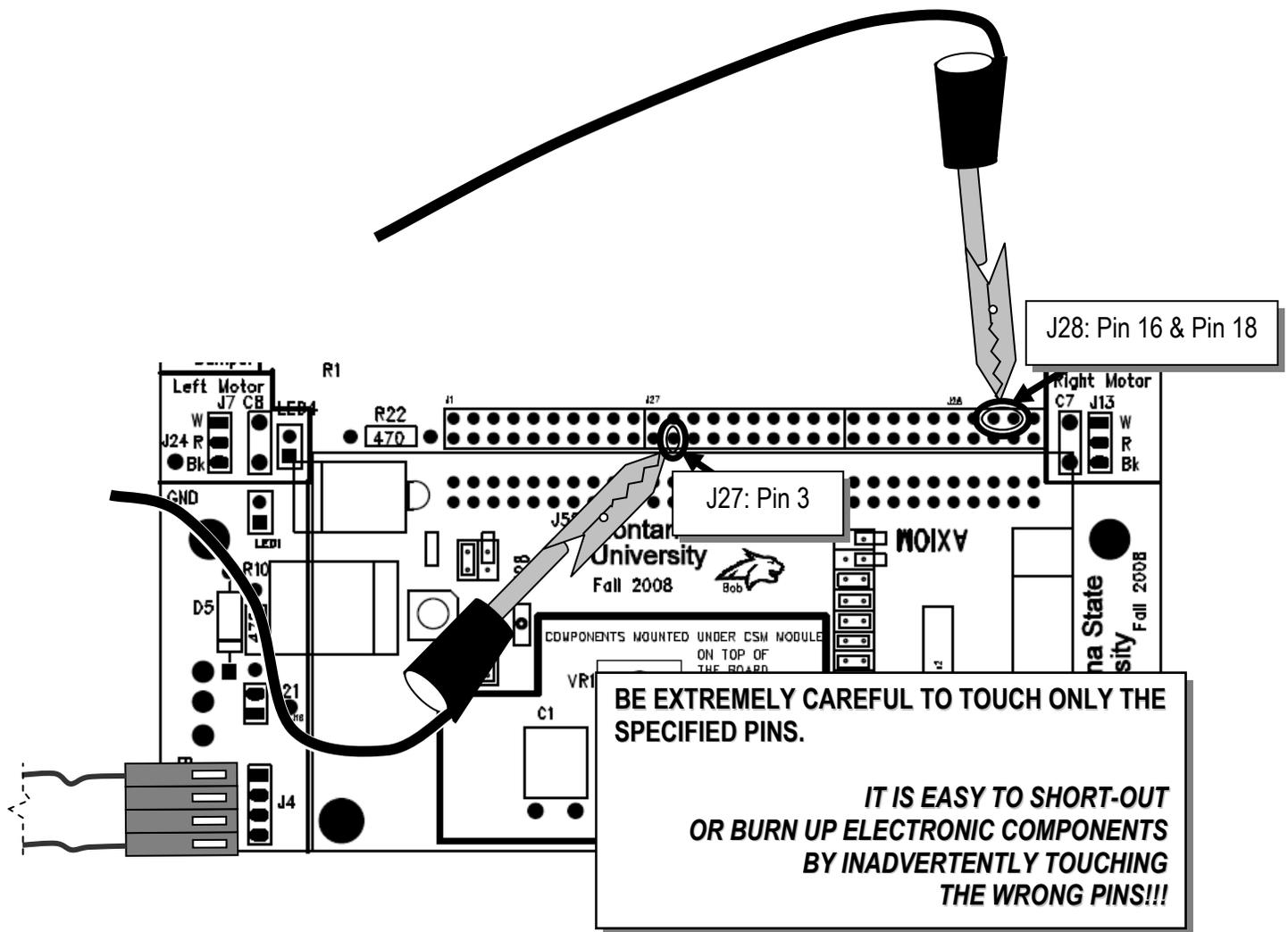
→ Finally, keep the grounded wire on J27 pin 3 and move the other grounded wire to J1 pin 19.
