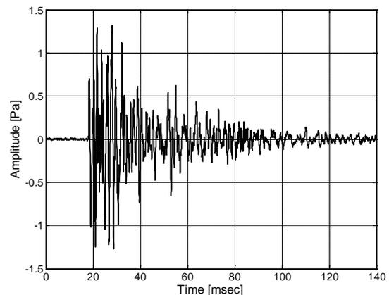
Figure 7: Recording of single gunshot, Glock 19 handgun, 9 mm ammunition. 24-bit, 48 kHz PCM, professional microphone inside closed vehicle, 7 meters from shooting position, 90° off-axis. Peak level 96 dB SPL re 20µPa
