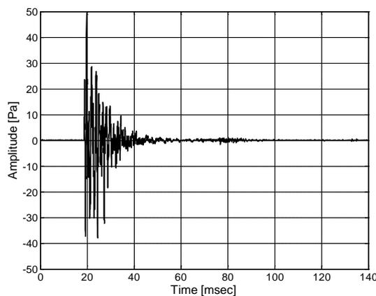
Figure 9: Recording of single gunshot, Glock 19 handgun, 9 mm ammunition. 24-bit, 48 kHz PCM, professional microphone inside open window vehicle, 7 meters from shooting position, 90° off-axis. Peak level 128 dB SPL re 20µPa.
