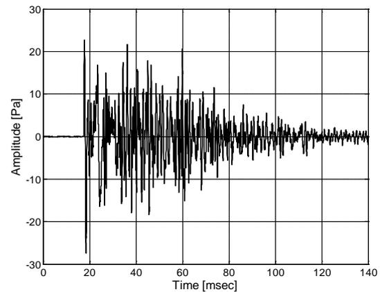
Figure 2: Reverberant recording of single gunshot, Glock 19 handgun, 9 mm ammunition. 24-bit, 48 kHz PCM, professional microphone at 8 meters, 90° off-axis. Peak level 123 dB SPL re 20  $\mu$ Pa.
