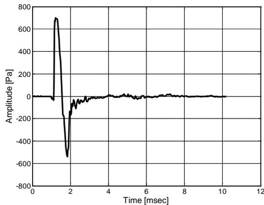
Figure 1: Anechoic recording of single gunshot, Glock 19 handgun, 9 mm ammunition. 24-bit, 48 kHz PCM, professional microphone at 3 meters, 9° off-axis. Peak level 151 dB SPL re 20  $\mu$ Pa.
