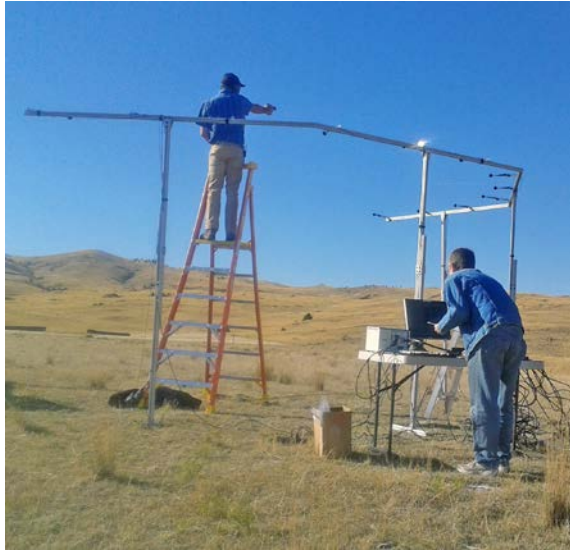
Figure 5: Handgun data collection using the multichannel recording system at the shooting range.
