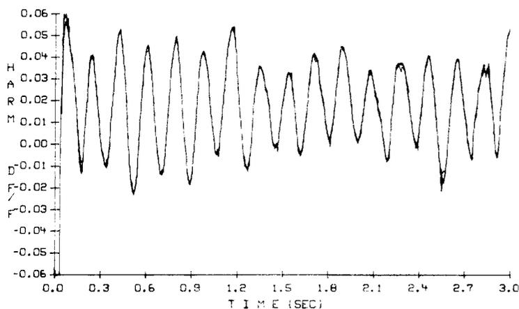
Fig. 6. Normalized measured frequency deviation for each of the partials of a typical alto tone, shown overlapped. Normalized deviations calculated by  $(f - kf_0)/(kf_0)$ , where  $f$  = measured frequency in Hz,  $f_0$  = assumed fundamental frequency in Hz and  $k$  = partial number ( $k > 0$ , integer).
