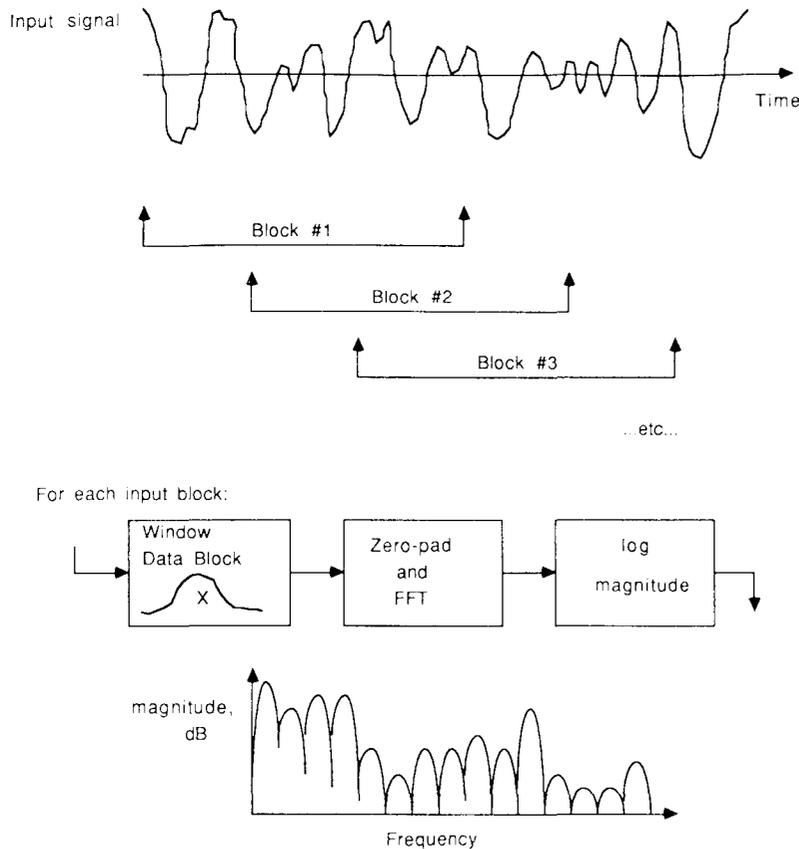
**Fig. 2.** Summary of the McAulay-Quatieri analysis procedure. The input signal is segmented into overlapping analysis blocks, or 'frames'. The log-magnitude spectrum of each block is computed, and the location and height of spectral peaks are identified.
