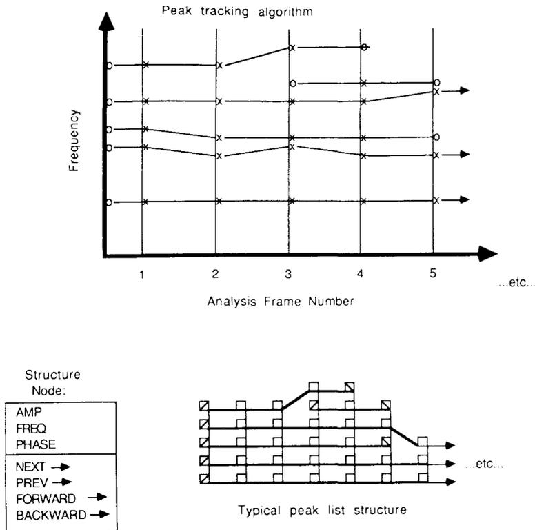
**Fig. 3.** The peaks from one analysis frame are connected with corresponding peaks in previous and subsequent frames. A data structure is constructed containing the amplitude, frequency and phase measured at each peak, and a set of pointers to each adjacent element (linked-list).
