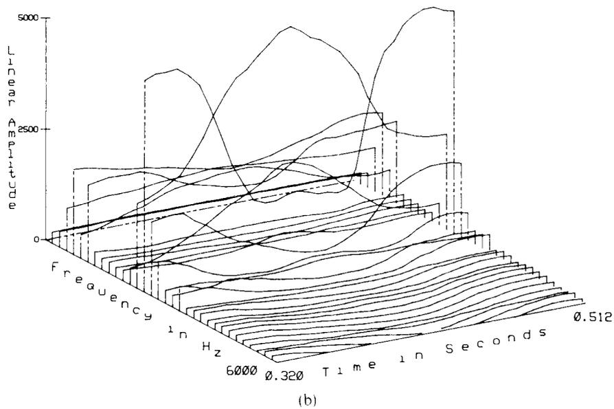
**Fig. 5.** Example of the conversion from a full MQ analysis to quasi-harmonic form. (a) A portion of the MQ analyzer output for a sung tenor tone. (b) The example of (a) following quasi-harmonic extraction based on fundamental frequency tracking.
