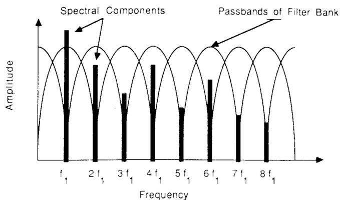
Fig. 1. A fixed-band harmonic analyzer employs a bank of bandpass filters centered at the harmonic frequencies. Vibrato causes the spectral components to shift back and forth in frequency, resulting in a misalignment ('cross-talk') between the analysis filters.
