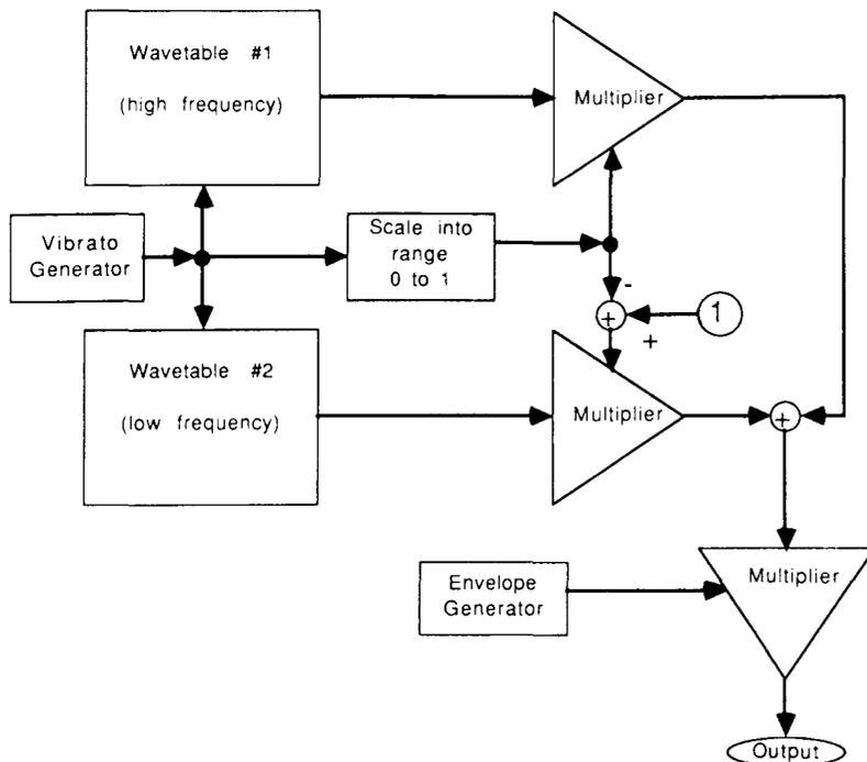
**Fig. 12.** Block diagram for panned-wavetable synthesis scheme. The contribution of each wavetable to the output is determined by the instantaneous vibrato extent. An overall amplitude envelope is applied to the signal.
