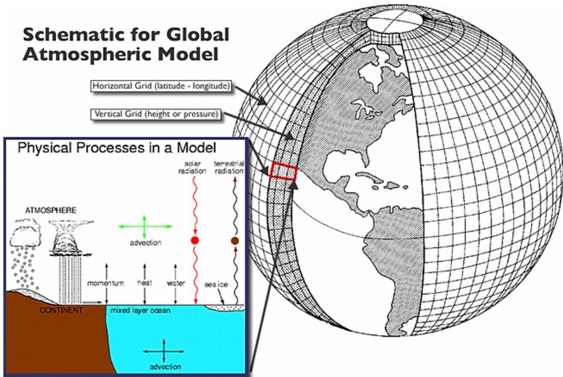
Climate models are systems of differential equations based on the basic laws of physics, fluid motion, and chemistry.
