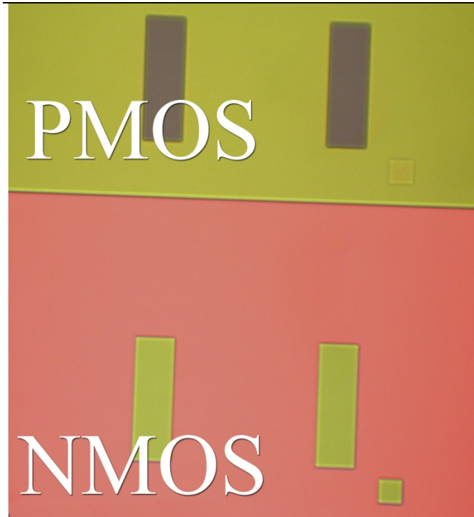
Figure 23 Diffused PMOS and NMOS sources and drains.
