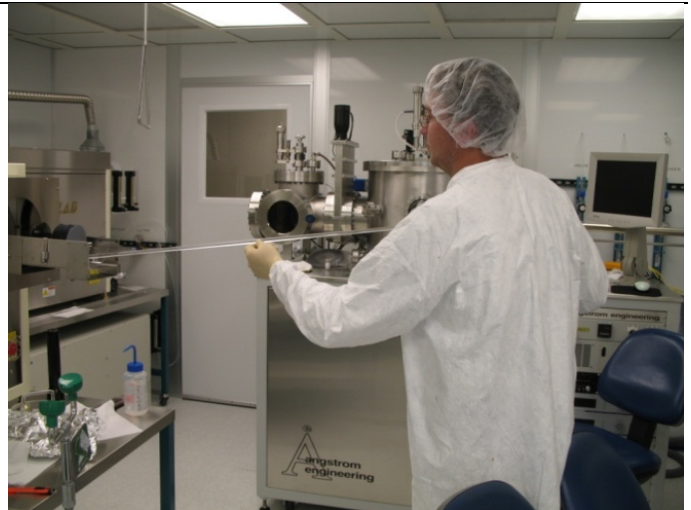
Figure 4 A student using a quartz rod to insert wafers into the oxidation furnace.
