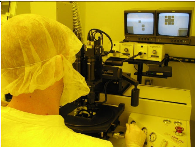
Figure 22 A student using the ABM mask aligner to align Mask #3.
