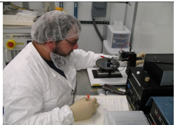
Figure 15 A student using the JANDEL 4-point probe to document the sheet resistivity of the diffusion.
